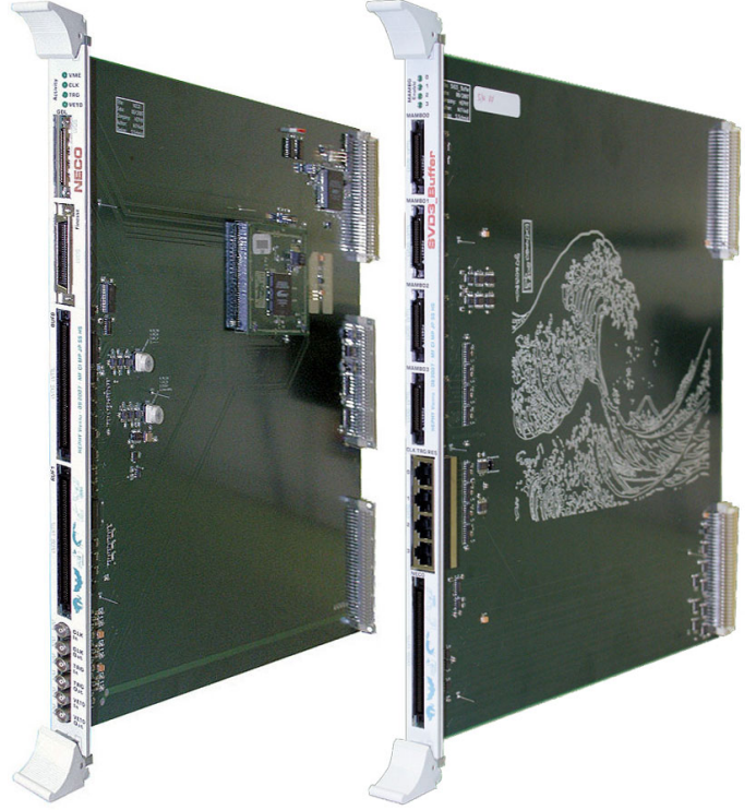
Figure 7: Control modules of the prototype system. The master control unit (NECO, left) is complemented by distribution units (SVD3_Buffer, right).
