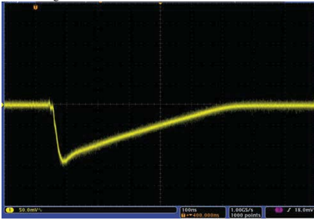
Figure 7 Measured Preamp response for a peak input current input of 250 \mu A with an input rise of 20ns and fall time of 450ns.
