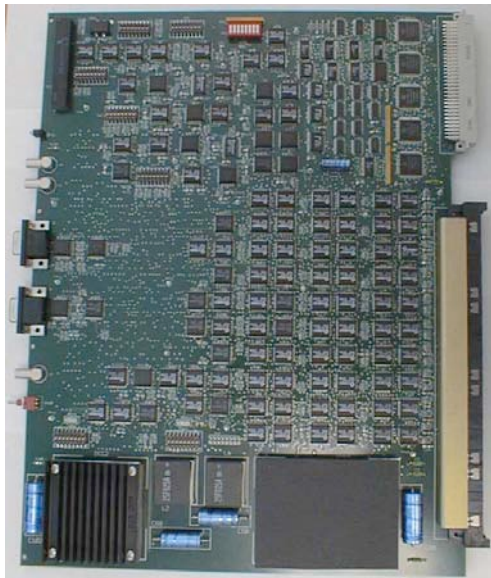
Figure 3. Pre-production Clock & Control Card.
