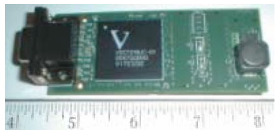
Figure 6. Close up of a pre-production 4 x 1.2 Gbit/s Copper receiver mezzanine card.
