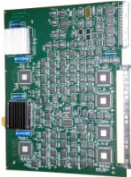
Figure 8. Pre-production Electron Isolation Card with Electron Isolation and Sort ASICs installed.
