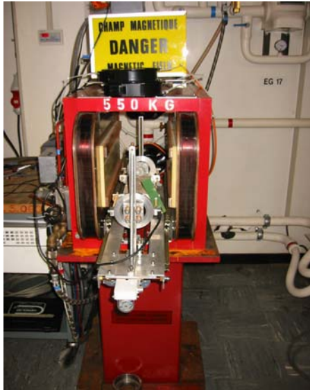
Figure 21 ESS test magnet (capable of 1.8kG).
