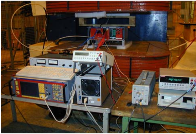
Figure 15 Device under test in the CMS-MNP2 magnet.
