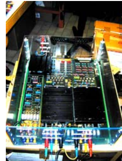
Figure 3: The dynamic load test fixture developed at Torino -INFN
