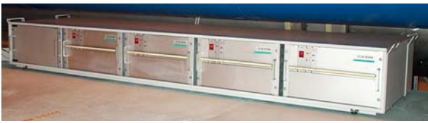
Figure 5: Quench Heater power supplies for the LHC main dipoles
