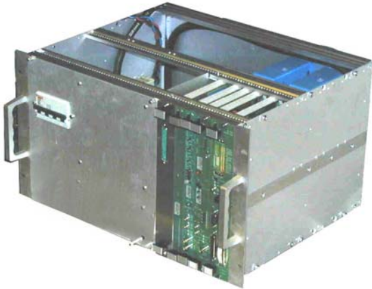
Figure 8: Powering Part for the LHC orbit corrector magnets at 60 A, \pm 8V
