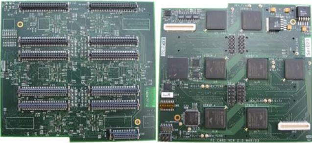
Figure 5: (left) Back side of the FE card; Connectors to the VFE cards and to the LVR card.
