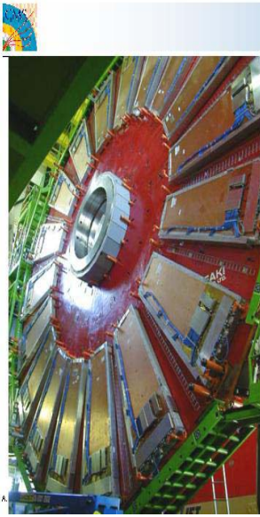
Fig.12- Cathode Strip Chambers of CMS for the muon detection in the forward region.
