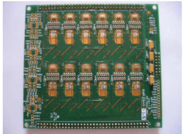
Figure 1: Hybrid which houses 12 chipsets consisting of two chips (known as ICON_4CH and VA4_PMT respectively)
