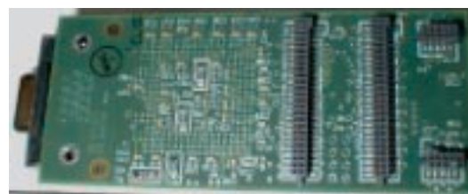
Figure 5. Pre-production 4 Gbit/s Copper Receiver Mezzanine Card.
