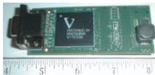
Figure 4. Pre-production Receiver Card rear showing Phase and Boundary Scan ASICs.
