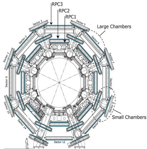
Figure 1: The ATLAS Muon Spectrometer Layout
