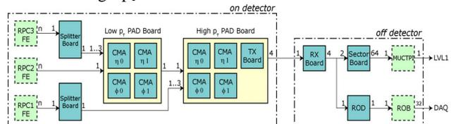
Figure 5: ATLAS Level-1 Barrel Muon Trigger Slice
