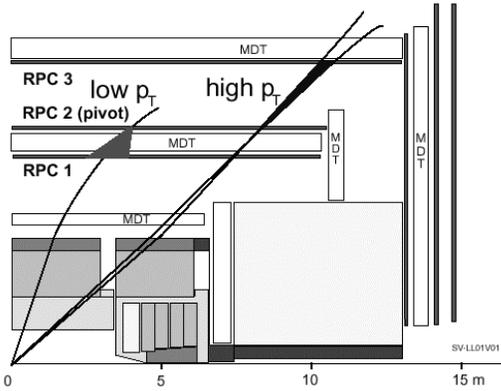
Figure 2: The ATLAS Barrel Level-1 Muon Trigger
