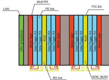
Figure 8: Off-detector crate with the contained VME cards
