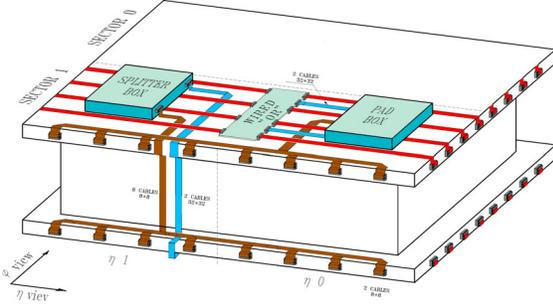
Figure 6: Schematic view of a Barrel Middle RPC station
