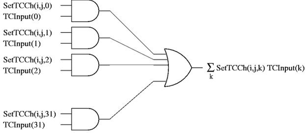
Figure 4: Tile Calorimeter coincidence implementation. For a given Pad and a given threshold a muon candidate is accepted if one hit is found in one of the corresponding Tile Calorimeter trigger towers.
