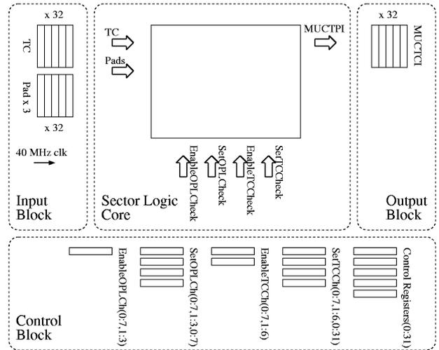
Figure 7: High level Sector Logic schematics with the interface with the test board. The Sector Logic core receives the input from the Input Block, the configuration parameters from the Parameters Block and sends its output to the Output Block. All the registers in the Input, Parameters and Output Blocks are accessible via the MFCC Power PC bus.
