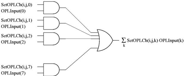
Figure 5: Low- $p_T$  filter implementation. For a given Pad and a given low- $p_T$  threshold a muon candidate is accepted if one hit is found in one of the corresponding RPC3 Pads.
