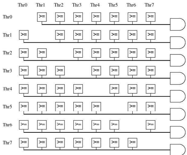
Figure 6: 1<sup>st</sup> highest threshold search implementation. For each Pad the muon candidate threshold is compared with the thresholds of all the other Pads and the comparison output are ANDed for each Pad.
