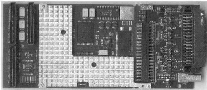
Figure 8: Layout of the MFCC with the FE adaptor card translating the MFCC Sector Logic output to LVDS logic levels used to interface the Sector Logic demonstrator with the MUCTPI prototype.
