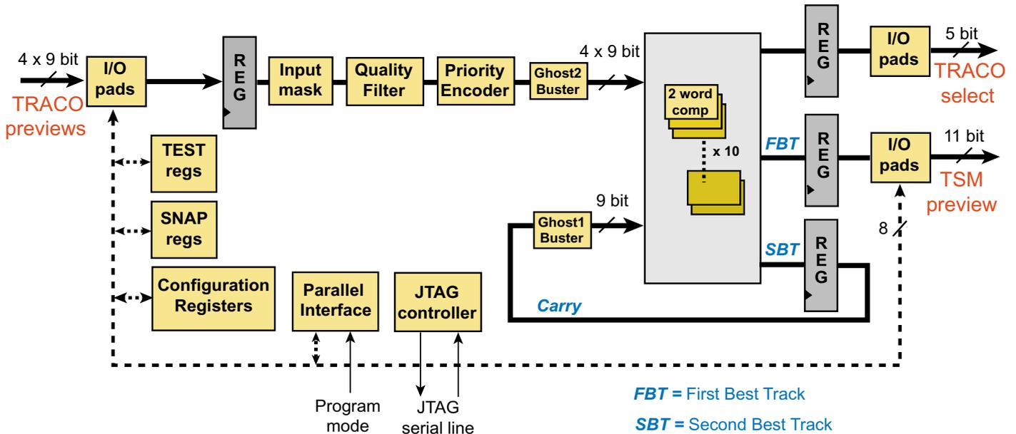
Figure 1: Block diagram of TSS functionalities.
