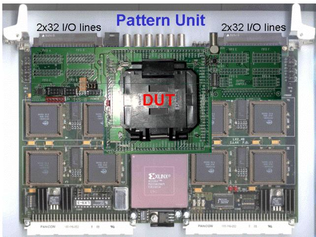
Figure 3: Pattern Unit hosting the DUT interface board.
