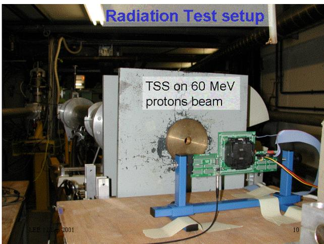
Figure 4: Radiation Test set up on 60 MeV protons beam. The test was made at the Cyclotron facility (CRC) in Louvain la Neuve (Belgium).
