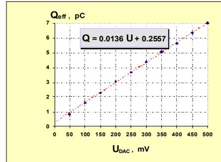
**Figure 6: Effective charge vs. DAC thresholds for 500 mV sweep of signals with fixed 1.6 ns FWHM and 0.9 ns equal edges.**
