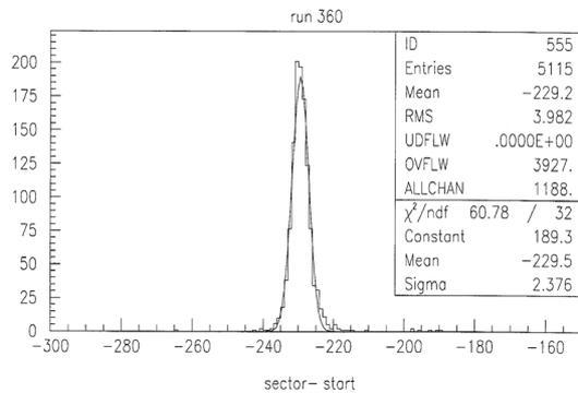
**Figure 11: Example of events over TDC channels distributions from the prototype MD tests at CERN PS (1 TDC channel = 50 ps).**
