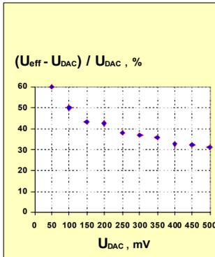
**Figure 4: Relative effective over DAC thresholds prevailing for 500 mV sweep of signals with 1.6 ns FWHM and 0.9 ns edges.**
