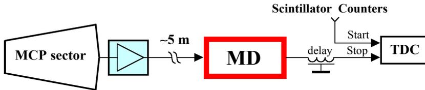
Figure 8: Experimental arrangement of the prototype MD tests with PS CERN / T10 setup facilities.
