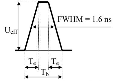
**Figure 5: Approximate shape of the generated pulse, indicating the quantities  $T_e = 0.9$  ns and  $T_b = 2.5$  ns.**
