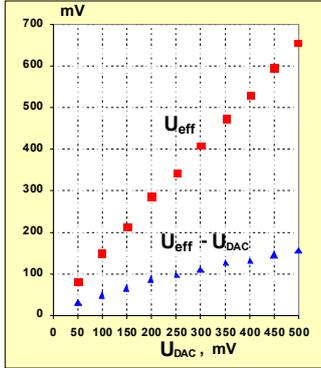
**Figure 3: Effective vs. DAC thresholds for 500 mV sweep of signals with 1.6 ns FWHM and 0.9 ns edges.**
