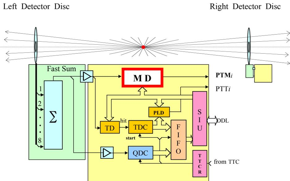
**Figure 1: General layout of the Multiplicity Discriminator (MD) within ALICE L0 Trigger Front-End Electronics (TTCR = the LHC Timing, Trigger and Control Receiver; TD = Time Discriminator; TDC = Time to Digital Converter; QDC = Charge to Digital Converter; PLD = Programmable Logic Device).**
