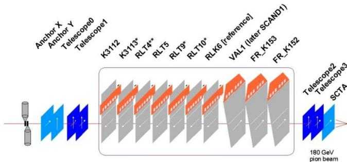
Figure 2: Sketch of the SCT experimental setup at H8 during August 2000. \*Barrel modules with irradiated detectors. \*\*Fully irradiated module, RLT4. Module RLK6 was used for reference, with fixed threshold and bias.
