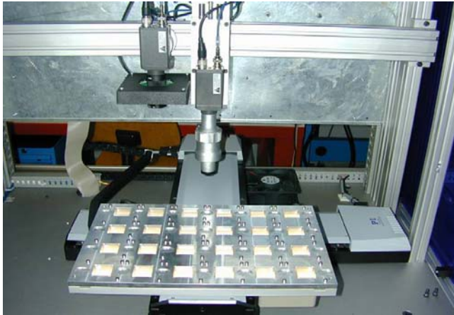
Figure 5: Optical scanning system (left) and chipcable detail (right).
