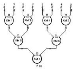
Figure 4: 8-channel passive summator of 2ns signal based on the UHF circular bridges application - general scheme
