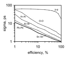
Figure 3: Timing resolution estimated for the case of relativistic nuclei collisions vs. start detector general efficiency.
