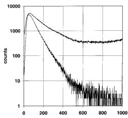
Figure 5: QDC spectrum: the sharmed beam test results of multiplicity registration with 5cm Pb target in front of the detector (upper curve) and empty target (low).
