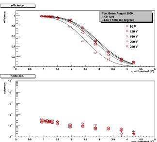
Figure 4: S-curves and noise occupancy in a 1.56 T field, normal incidence for unirradiated barrel module K3112 at all detector bias values studied.
