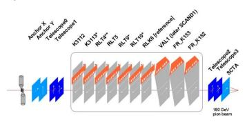
Figure 2: Sketch of the SCT experimental setup at H8 during August 2000. \*Barrel modules with irradiated detectors. \*\*Fully irradiated module, RLT4. Module RLK6 was used for reference, with fixed threshold and bias.
