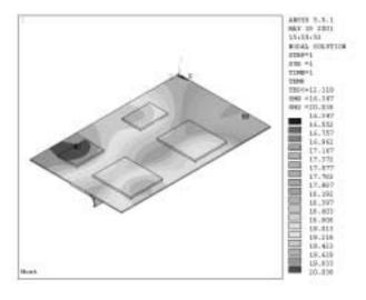
Figure 4: ANSYS simulations of the carbon fibre SDD heat bridge temperature map for the uniform conductivity 180W/(mK)
