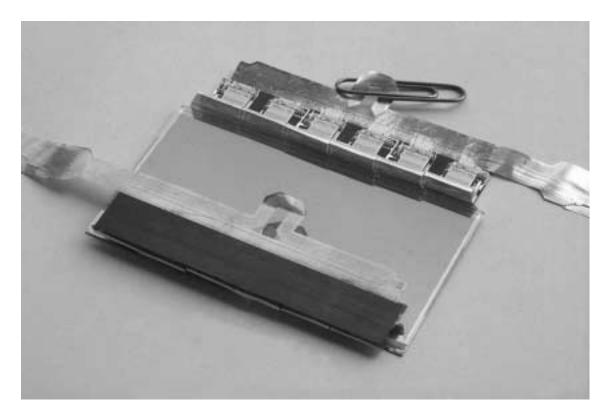
Figure 6: Foto of the SDD detector for ALICE ITS equipped with real CF hybrids with chips and microcables mounted
