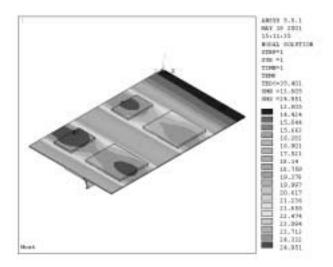
Figure 3: ANSYS simulations of the carbon fibre SDD heat bridge temperature map for the undirectional fibre orientation. Position of the thermoconductive clip is optimised
