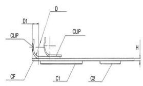
Figure 5: SDD CF motherboard with chips, Side view: CF-carbon fibre motherboard; C1,C2 - FEE SDD chips (Ambra and Pascal); D1=2mm,D=1,9mm;H=240microns. Length of the CF SDD board =65mm, width=20mm
