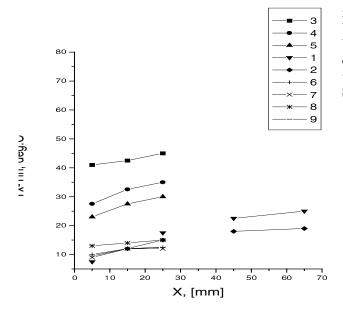
Figure 2: Temperature distributions along the tested heat bridges obtained under 2 W heat load (except samples No.1 and 2 tested under 1W load). Copper bridge No.1 (see Table 2) has an ideal (soldered) contact with the cooling tube fixed to one side end of the bridge.
