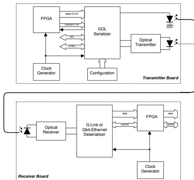
Figure 2 : Test setup block diagram
