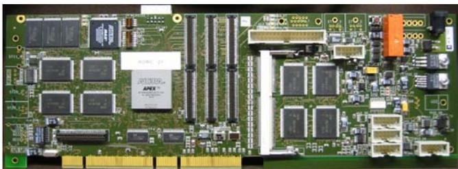
Figure 3: The prototype of the HLT-RORC.
