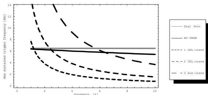
Figure 5: sustained trigger frequency for MEB and DDL.
