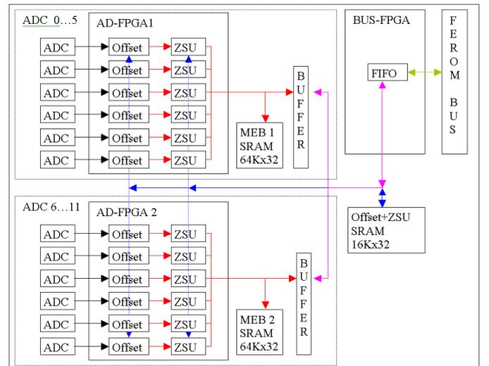
Figure 3: AD-module architecture
