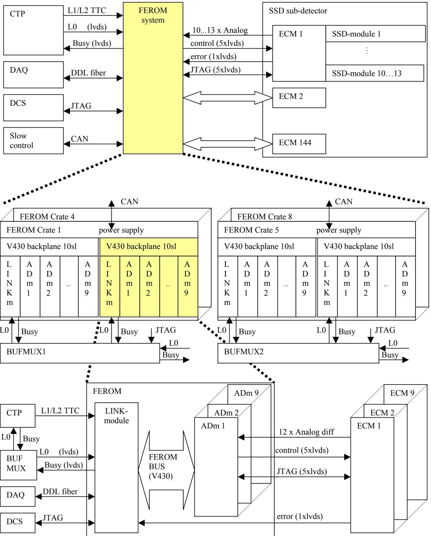
Figure 4: FEROM system interface, partitioning and architecture
