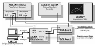
Figure 2 : The test platform
