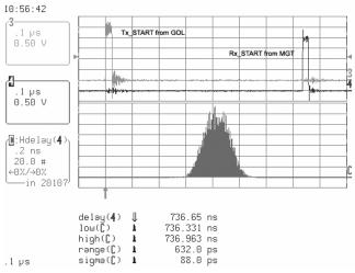
Figure 8 : Latency delay distribution in the synchronous mode. The Gaussian shape, of this jitter, characterizes a pure random source.
