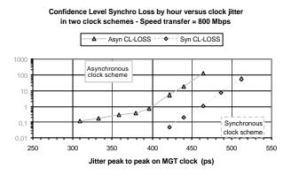
Figure 6 : Synchronization loss measurements
