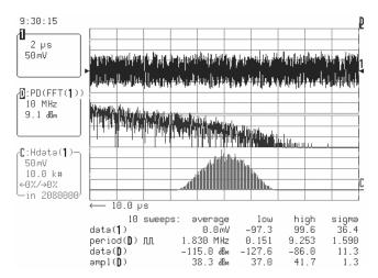
Figure 3 : Injected noise analysis. The upper waveform gives the time domain The middle one show the frequency domain (Power Distribution with a FFT) and the lower one depicts the Probability Density Function (PDF) of the noise which as expected has a Gaussian shape.
