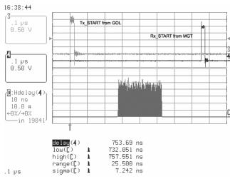
Figure 7 : Latency delay distribution in the asynchronous mode
