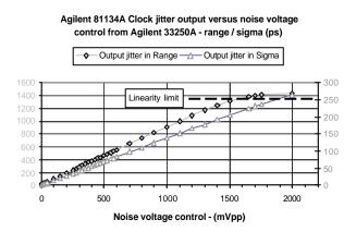
Figure 4 : Transfer function of the pulse/pattern generator. The left/right vertical scales give the jitter range (ps) and the jitter sigma dispersion (ps).
