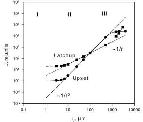
Figure 4. Typical dependences of threshold energy on local spot radius
