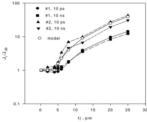
Figure 2: Normalized laser threshold energy as a function of laser spot for two pulse duration and for the first and the second structures
