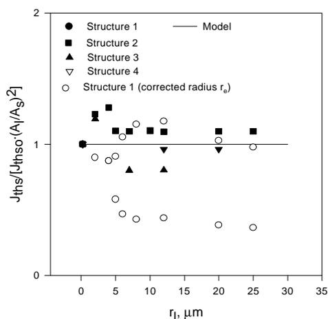
Fig.6. Relative upset threshold energy as a function of laser spot radius (computer simulation)
