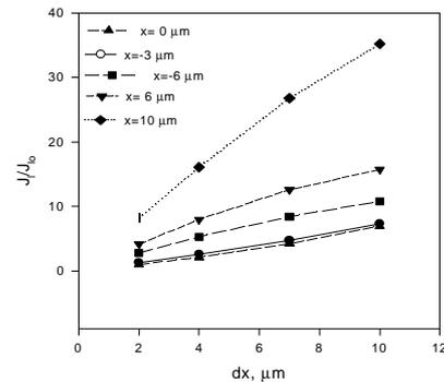
Figure 1: Latchup threshold energy as a function of stripe width and its location
