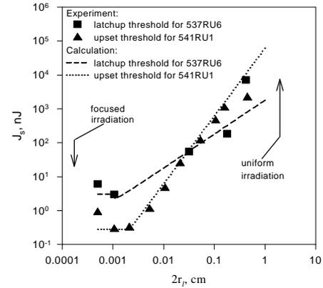
Figure 3. Experimental data of latchup and upset laser threshold energy vs. laser spot diameter for 541RU1 and 537RU6
