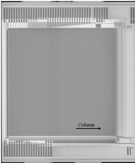
Figure 3. Photo of the 512x512 sensor. Columns are oriented horizontally in this picture. On the right, i.e. at the bottom of the columns, adjustable gain column amplifiers together with a 10-bit ADC per column.
