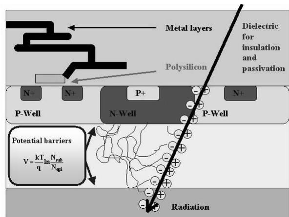
Figure 2. Schematic view of the cross-section of a CMOS process.
