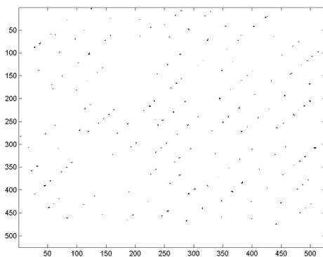
Figure 5. Raster scan with 140 keV electrons recorded with the 512x512 device. The beam was set so that each spot carried an average of 2 electrons per spot. Because of Poisson statistics, this means that some spots will have no electron. The distribution of electron per spots fits well with the expected Poisson distribution.
