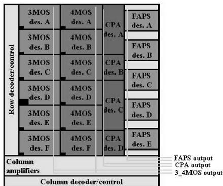
Figure 7. Floorplan of the parametric test sensor.
