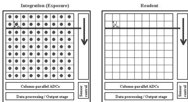
Figure 1. A commercial sensor normally operates in two sequential phase, the integration (on the left) and then the readout. While the integration can be done either in the rolling shutter mode (row by row) or in the snapshot mode (all pixels at the same time, the readout is always done row by row).
