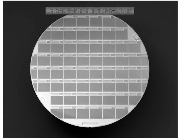
Figure 6. Photograph of the 200 mm wafer with the three sensors designed in a 0.25  $\mu\text{m}$  CIS process. In each reticle, the large sensor is the 3k\*4k sensor. On top of this, on the right is the linear sensor and of the left is the parametric test sensor.
