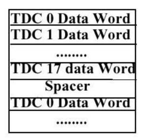
The spacer word will have a 4 bit code and 18 parity bits, one for each previous 18 data word.
