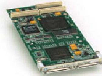
Figure 5: Photo of Dolphin SCI card (PMC version). SCI packets are received and transmitted via two 16 bit wide differential LVDS connectors. The PCI mezzanine connectors are configured for 64 bit and 66 MHz.
